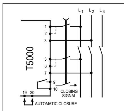
Fig. 1. Connection Diagram.
